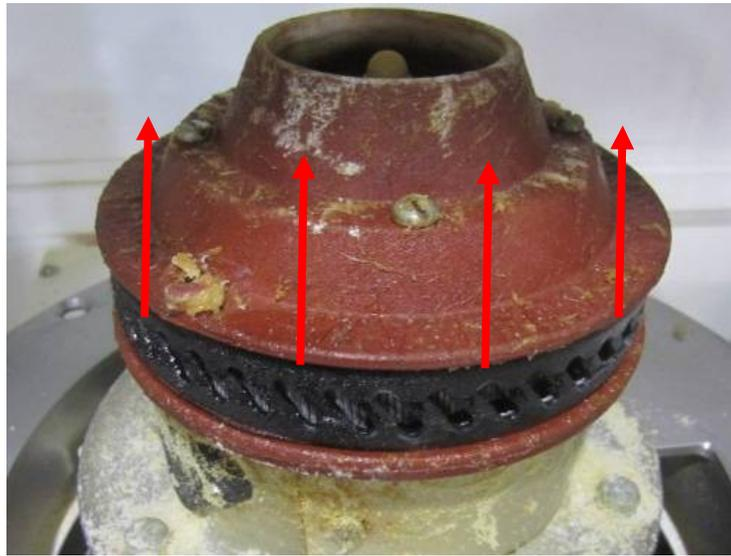
※ When installing the heater, make sure the 4 brushes fixed on brass tracks or it may cause the heater to get shorted and damaged.
