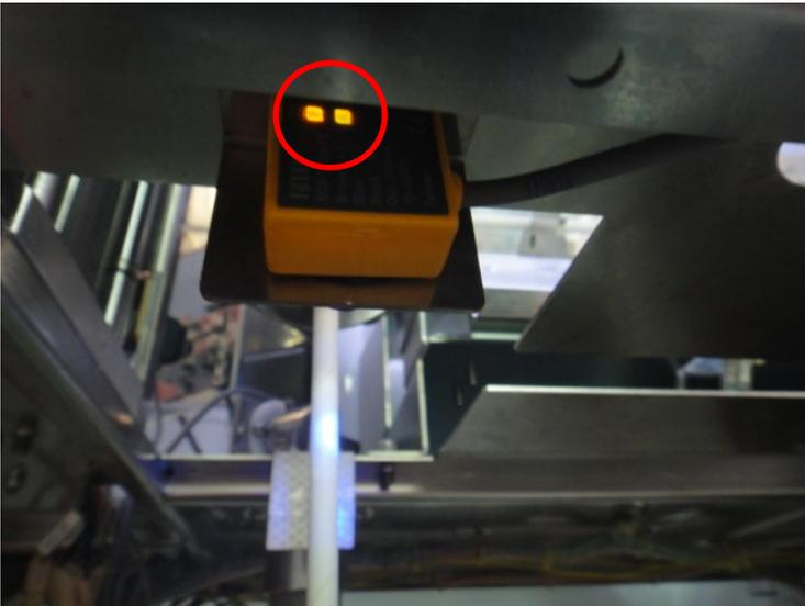
(C) The stick sensor shines blue light on reflecting sheet. Make sure the blue light shoots toward the sheet properly. The blue light is also the range of sensor detecting. If it is out of adjustment, loosen 2 screws on sensor bracket and then adjust its shooting position.
